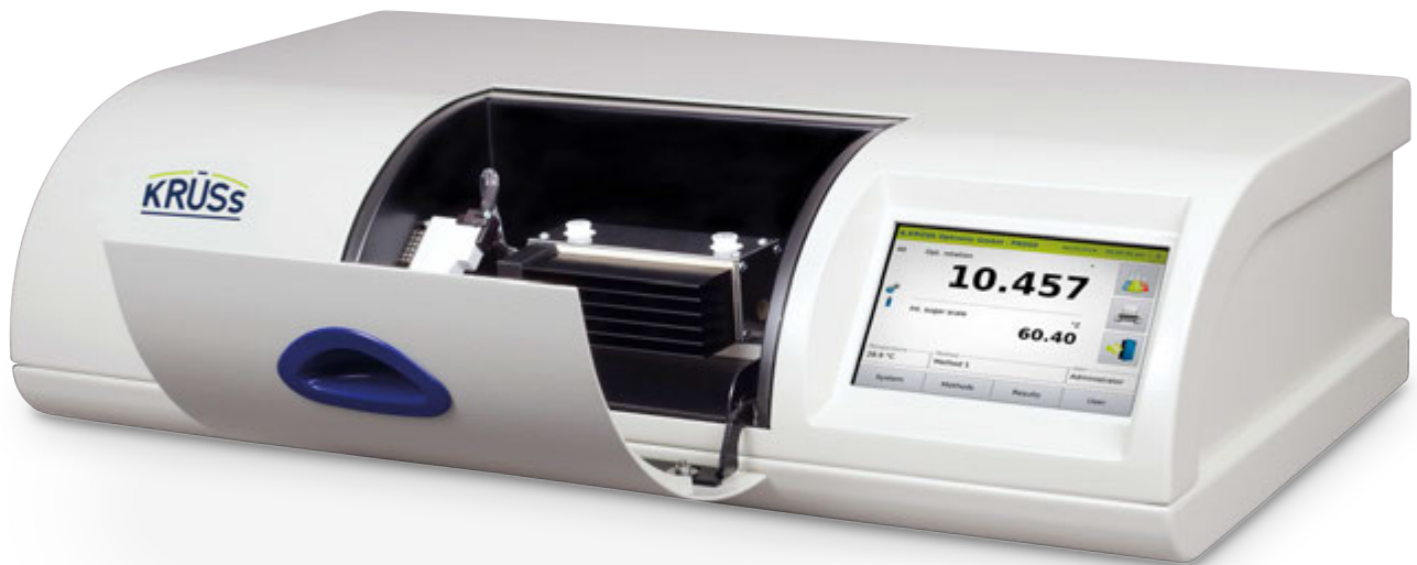
P8000-P with measurement tube PRG-100-EPT
