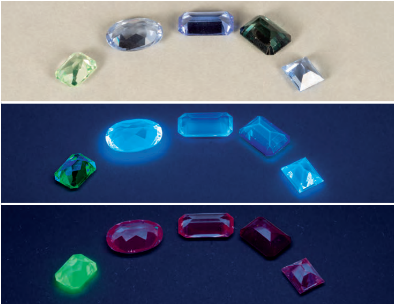
Fig.29: Green and light blue synthetic spinels under artificial light (top row), long-wave (middle row) and short-wave (bottom row) UV light. In their fluorescent colour, all stones exhibit a distinctive colour change under UV light of different wavelengths.
